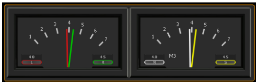
Example: PPM display in Dual L/R mode left beside Dual M/S mode with horizontal orientation of TM3-3G Smart
