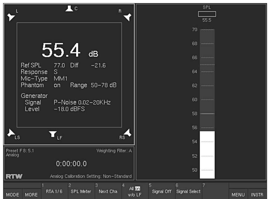
Fig. 5-26: First Toolbar function layer of the CAL instrument. Select MORE to display additional functions (layer 2)
