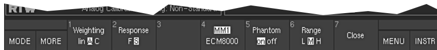
Fig. 5-34: Screen display after selecting the SPL Meter function of the CAL instrument's second function layer
