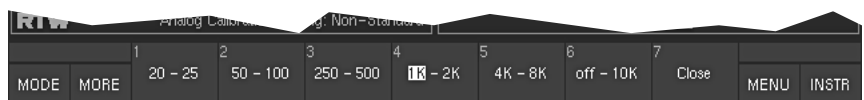
Fig. 5-33: Second Toolbar function layer of the Sine test signal (displayed after selecting MORE)
