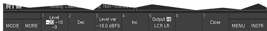
Fig. 5-30: Screen display of the first function layer of the LF-Test signal. Select MORE to display additional functions (layer 2)
