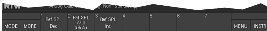
Fig. 5-27: Second Toolbar function layer of the CAL instrument (displayed after selecting MORE)
