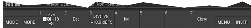
Fig. 5-32: Screen display of the first function layer of the Sine signal. Select MORE to display additional functions (layer 2)
