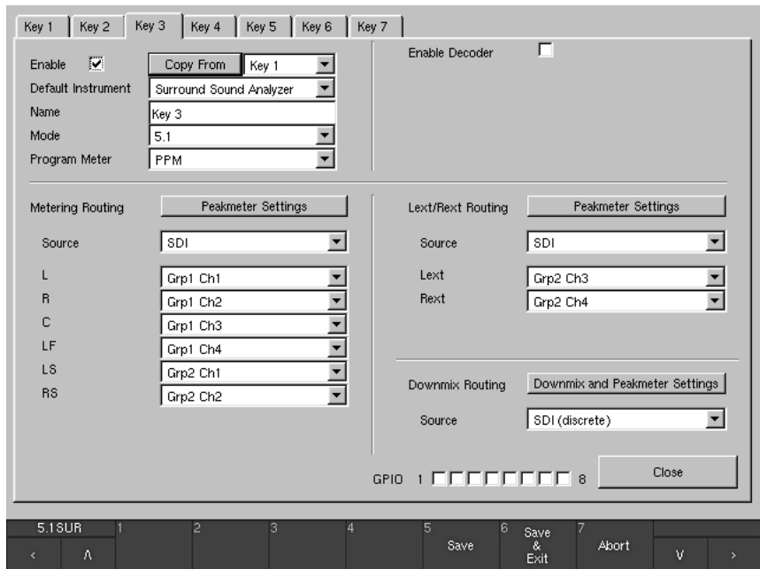
Fig. 3-11: The Key 1 to 7 Sub Preset menu tabs of the Input Routing setting
