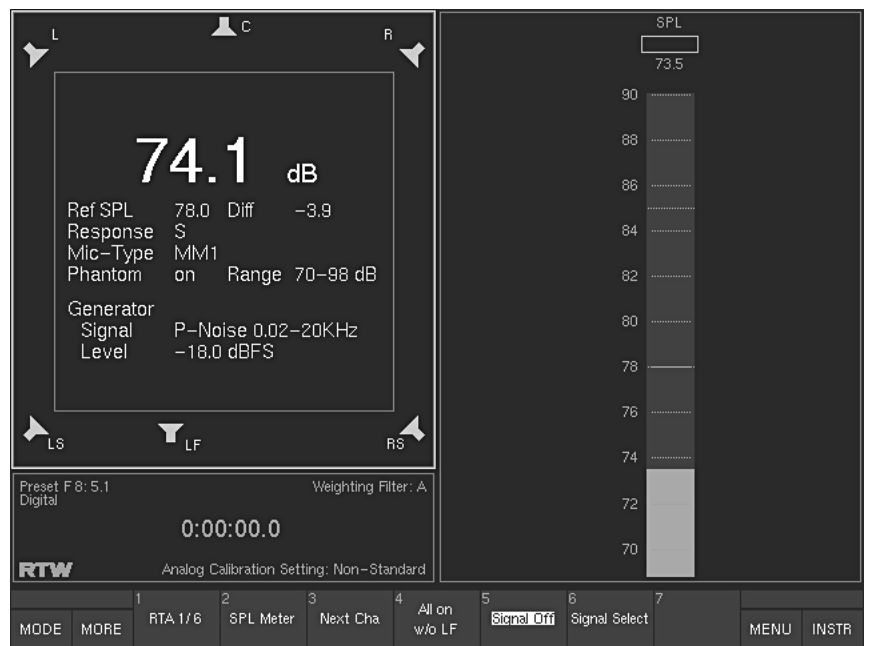
Fig. 2-10: The calibration instrument (CAL) displayed in window 3 (highlighted with a white frame)
