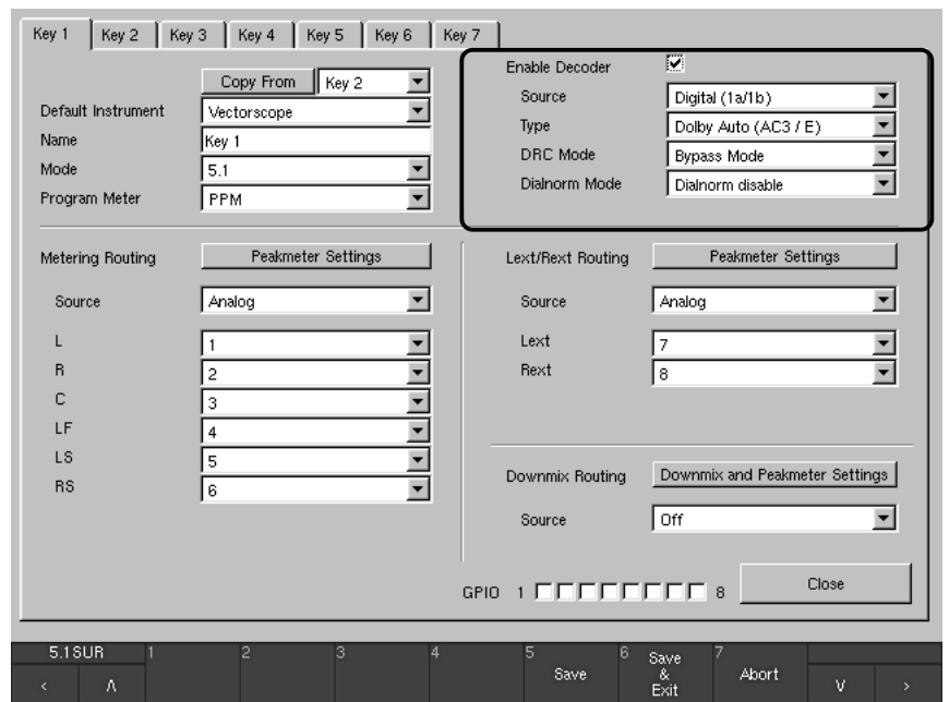
Fig. 6-27: Example for the enabled Dolby® decoder (only with D and SD versions)
