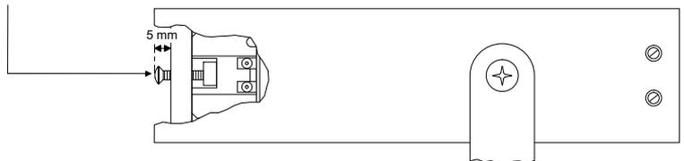
3) Grasp the two screws and pull the instrument out of the case 1020E respectively out of the 19"/1U rack mount kit (with mounted bracket 1128H).
