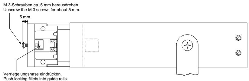
4) Slide the instrument into the case 1020E respectively into the 19"/1U rack mount kits (with mounted bracket 1128H) and fasten it with the two Philips screws.
