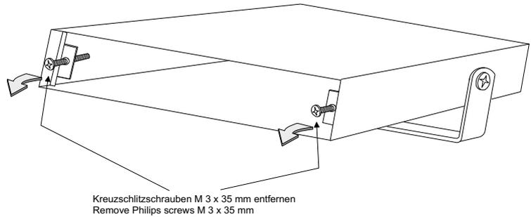
2) Loosen the Philips screws at the front panel of the instrument until they protrude by about 5 mm of the front panel.
