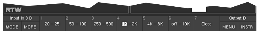
Fig. 3-23: Second Toolbar function level of the SINE instrument (displayed by selecting MORE)
