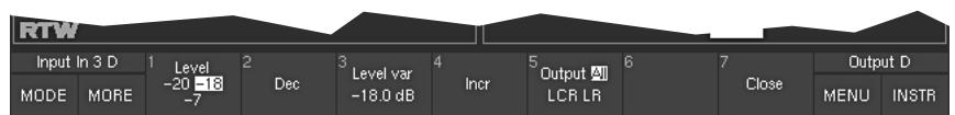
Fig. 3-20: First Toolbar function level of the LF-TEST instrument. Select MORE to display additional functions (level 2).
