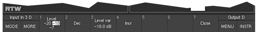
Fig. 3-22: First Toolbar function level of the SINE instrument. Select MORE to display additional functions (level 2).
