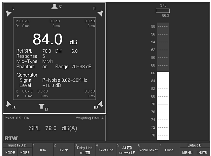
Fig. 3-16: First Toolbar function level of the CAL instrument. Select MORE to display additional functions (level 2).
