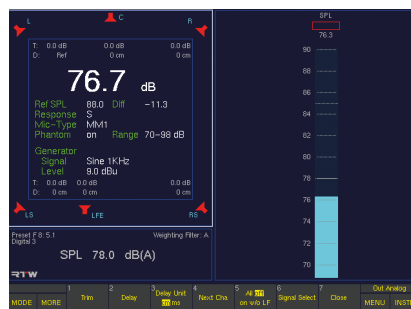
The Surround test signal generator in calibration mode
