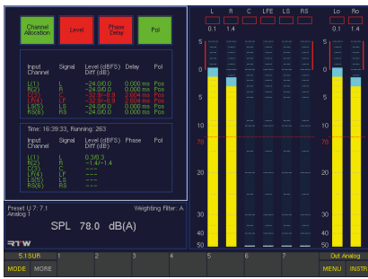
BLITS generator and extended BLITS analyzer
