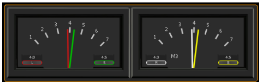
Example: PPM display in Dual L/R mode left beside Dual M/S mode with horizontal orientation of TM3 Smart
