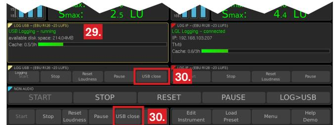
30. Touch the key labelled with **USB close** to stop collecting the logging data, to store them on the connected USB flash drive and to close the logfile. While this procedure is running, the red-colored status message „USB Logging – busy“ is displayed in the top line of the Logging instrument.
