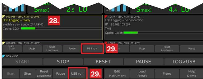
29. Touch the key labelled with **USB run** to start logging data into a logfile on the connected USB flash drive. While this procedure is running, the green-colored status message „USB Logging – running“ is displayed in the top line of the Logging instrument.
